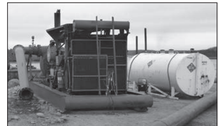
Inline booster pump pushes slurry far down the beach. Diesel tank (right) is filled daily when the machines are running.
